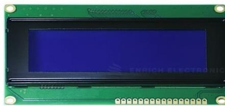
**Gambar 2.3 LCD 20x4**
