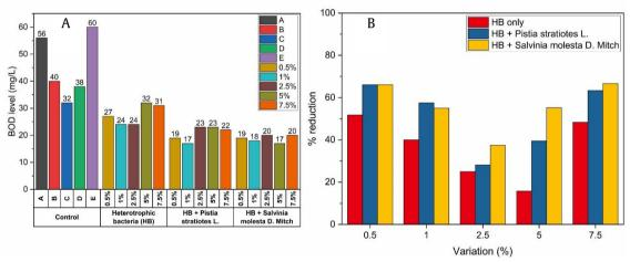
Figure 2. (A) BOD 5-day test result and (B) effect of each treatment on BOD level
