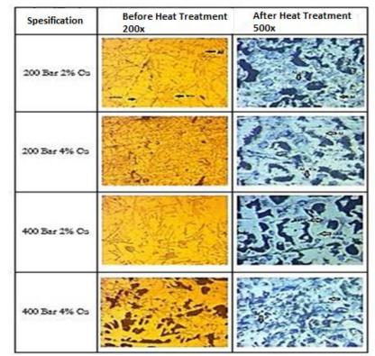
Table 2. Microstructure observation of before heat treatment of 2% and 4% cu composition
