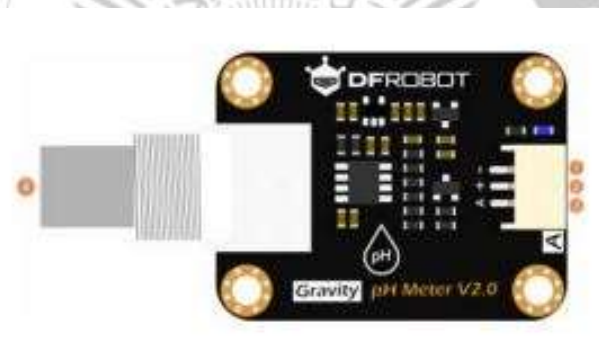
Gambar 2.2 Modul Signal Conversion Board (Transmitter) V2
