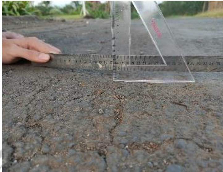
Gambar 4.6 Kedalaman Bekas Roda STA 1+900 – 2+000
