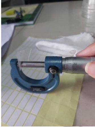
Pengujian Ketebalan Edible film
