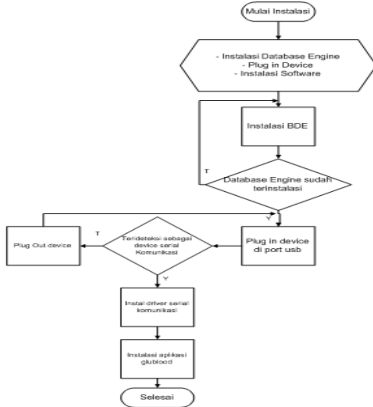
Gambar 2 Diagram alir Sistem Monitoring
