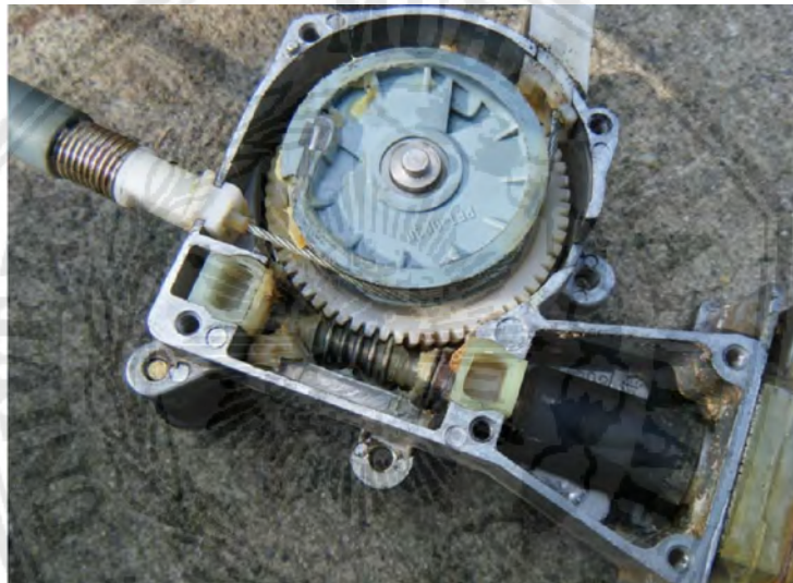
Gambar 2.3 gear vertical to horizontal power window
