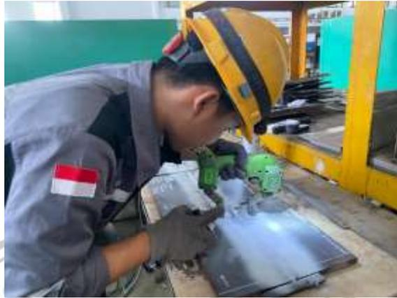
**Gambar 3.13** Proses Inspeksi *Magnetic Test*
