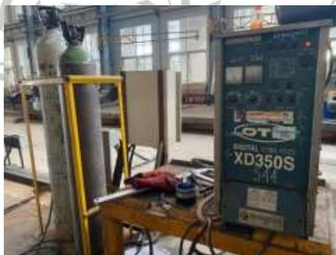
**Gambar 3.7** Mesin Las Gas Metal Arc Welding
