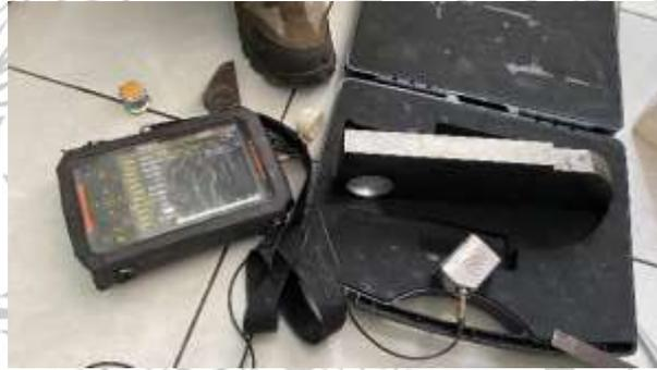
**Gambar 3.14** Kalibrasi *Ultrasonic Test*
