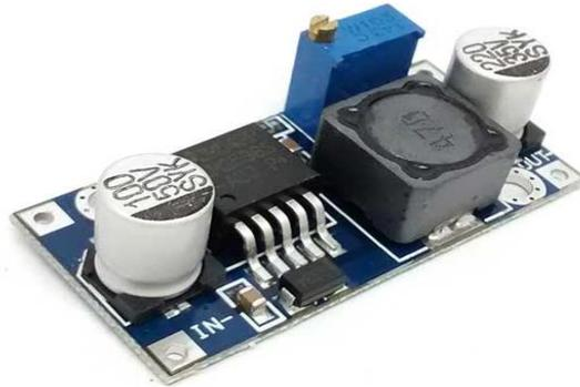
*Gambar 2.13 LM2596 DC-DC Step Down*
