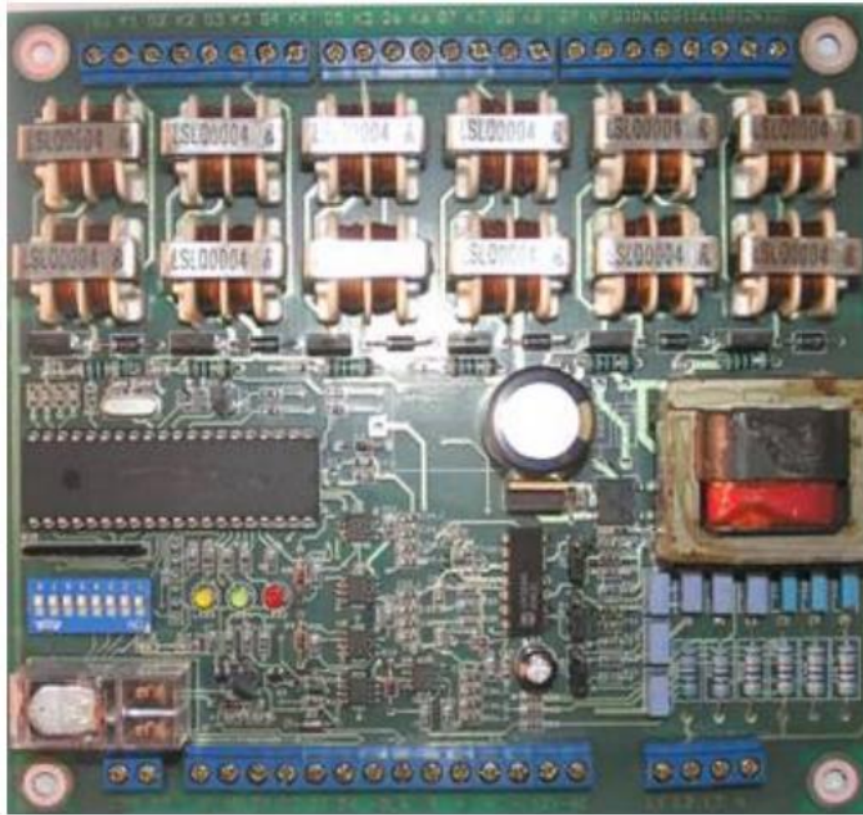
Gambar 7.21. Mainboard kontrol PLTMH Sengkaling 1-UMM (Sumber : Renerconsys, "Standard Operasional Digital Load Controller PLTMH UMM", 2009)
