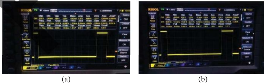
FIGURE 8. (a) Photo of measurement results at a period of 10 ms and T_{on} on 1.5 ms, (b) Photo of measurement results at a period of 10 ms and T_{on} on 1.8 ms
