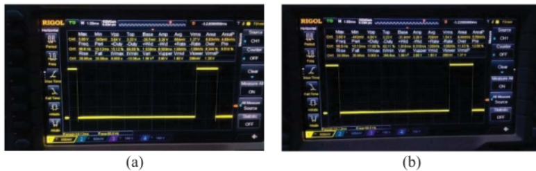
FIGURE 8. (a) Photo of measurement results at a period of 10 ms and T on 1.5 m, (b) Photo of measurement results at a period of 10 ms and T_on 1.8 ms
