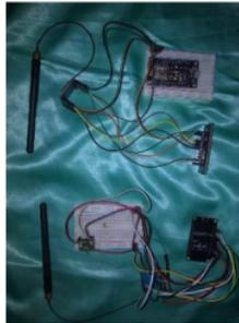
Gambar 7. Lora Ra-02 Transmitter dan Receiver
