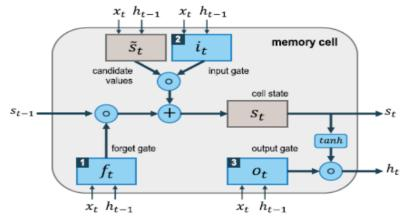
Figure 1. The LSTM network architecture memory cell [15]
