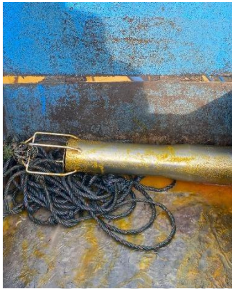
Gambar 13. Alat bacon bomb sampler
