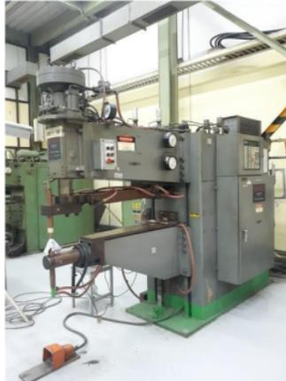
**Gambar 2** Mesin *Resistance Spot Welding* SCIAKY Tipe P272
