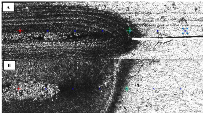
Gambar 8 Skema Pengindentasian Uji *Micro Hardness*
