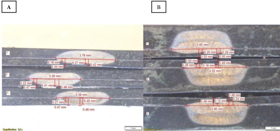
**Gambar 7** *Macrography* Weld Nugget Spesimen Uji
