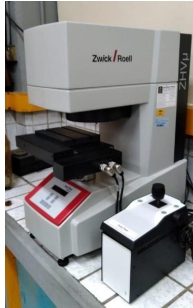
Gambar 5 Mesin Zwick Roell ZHV \mu Micro Hardness Tester
