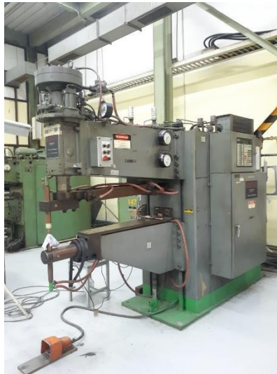
Gambar 2 Mesin Resistance Spot Welding SCIAKY Tipe P272
