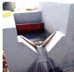
triangle threshold downstream of the piping
