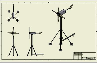
FIGURE 4. Wind Turbine Design
