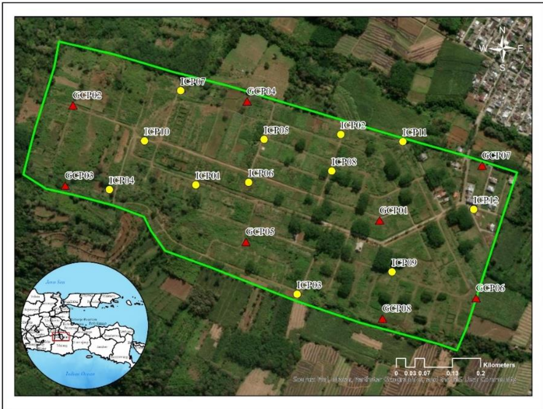
Fig. 3. Control points configuration in the study area. Red triangles represent GCPs, yellow circles are ICPs, and green lines represent areas of interest.
