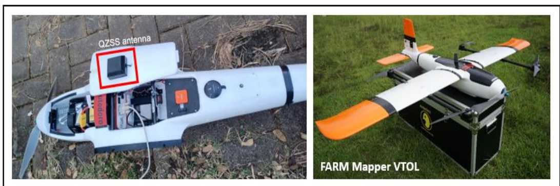
Fig. 2. QZSS antenna installation on Fixed-wing UAV.
