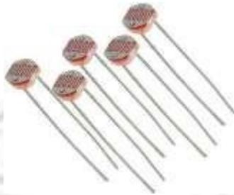
**Gambar 2.3** LDR (Light Dependent Resistor)
