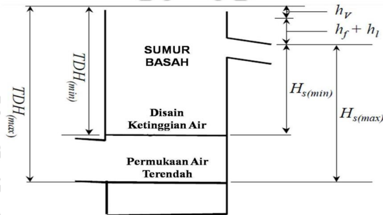
Gambar 4. 4 Ilustrasi perhitungan TDH (Total Head Dynamic)
