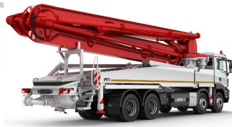
Gambar 2.4 Concrete Pump Truck
